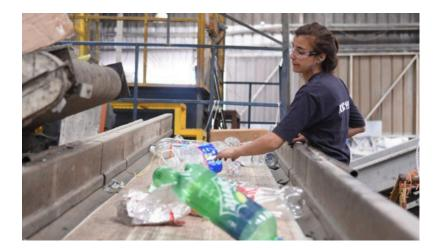
**Dirty materials:** A mixed waste processing system accepts a stream of mixed solid waste and then proceeds to separate the designated recyclable materials through a combination of manual and mechanical sorting. Sorted recyclables may undergo additional processing necessary to meet technical specifications set by end markets, while the remainder of the mixed waste stream is sent to a disposal facility, such as a landfill.
