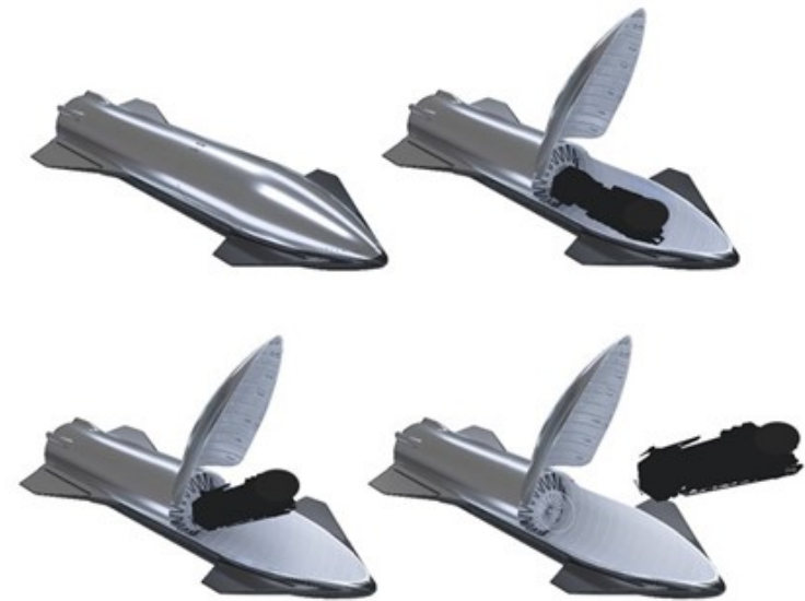
Figure 3: Starship payload deployment sequence
