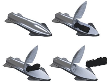
Figure 3: Starship payload deployment sequence
