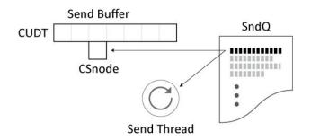
The SndQ is a double link list, where each entry points to the send node (CSnode) of a send buffer. CSnode is an object of the SndQ class (SndQ is a queue, but there are other members in the class). CSnode is not related to the buffer contents. It has a pointer to its socket, timestamp and a location (where it was inserted in the SndQ).
