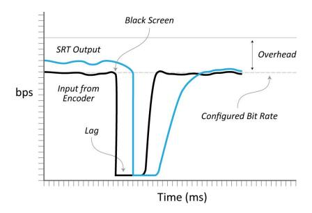
To correct this, the SRT sender's output can be configured at the nominal bit rate of the input by interacting more directly with the video encoder on which SRT is running. Since it is possible to know the bit rate at which the encoder is configured, any modification can be passed directly into the SRT configuration (INPUTBW). This is the goal.
