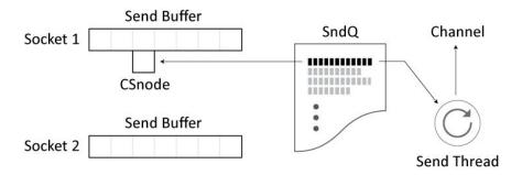
Each packet has a timestamp that dictates when to send it. The SndQ List is sorted in order of the timestamps to be processed. If the send thread determines that the socket 1 send buffer has a packet ready, then it adds it to the SndQ queue. If the SndQ queue is empty, the packet entry is placed at the beginning, with its timestamp, which determines when the packet needs to be processed.
