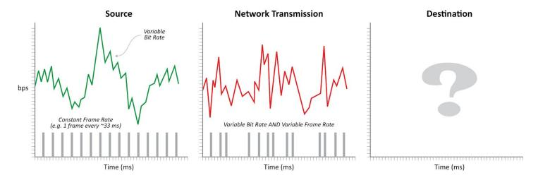
SRT includes a mechanism that recreates the signal characteristics on the receiver side, dramatically reducing the need for buffering. This functionality is part of the SRT protocol itself, so once data comes out of an SRT connection on the receiver side, the stream characteristics have been properly recovered.
